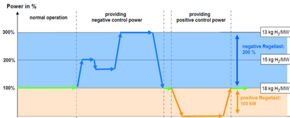
Figure 4: Example for capabilities of PEM electrolyzers for hydrogen production in DSM systems [Waidhas 2011]
